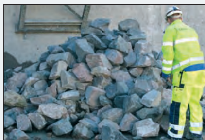
Figures 15 and 16 - Schematic sketch of rock crushing area in front of the cutterhead and typical blocks passing through the cutterhead openings.
