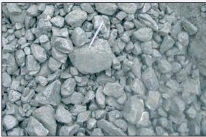
Figure 18 - Typical tunnel muck from closed mode operation (rounded blocks).
